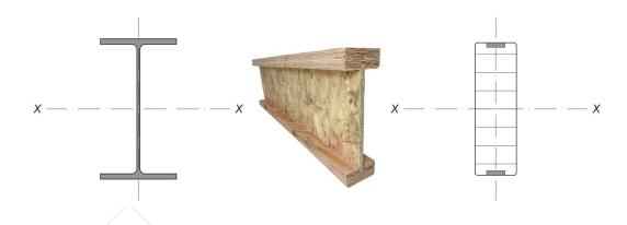
Bending stiffness, aka flexural rigidity, is directly related to the second moment of inertia I of a beam's cross-section.
